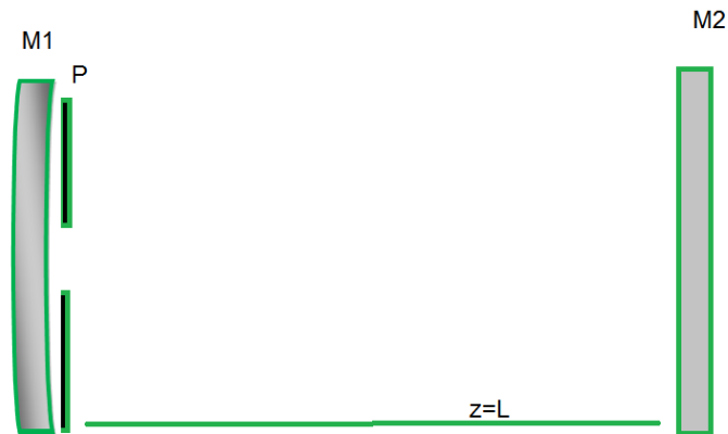
Figure 3.1: Simple cavity resonator system
