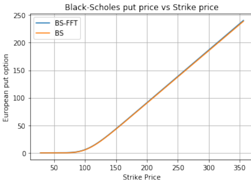
Figure 3.3: Comparison of the Black-Scholes analytical solution vs FFT for European put options.
