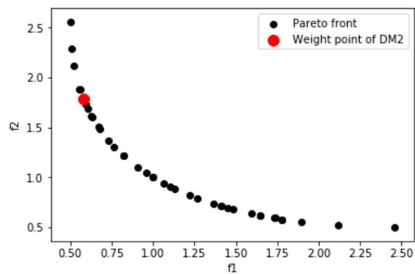
Figure 3.3: A Pareto front for the given functions. The red point is the point which obtained from the weight of decision maker two.
