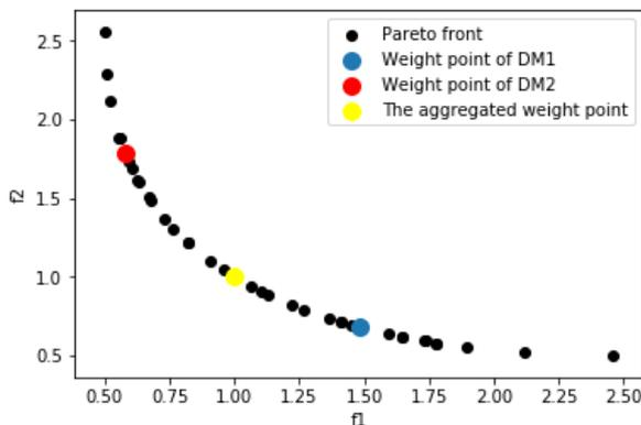
Figure 3.4: A Pareto front for the given functions. The yellow point is the point which is obtained from the aggregated weight.
