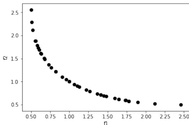
Figure 3.1: A Pareto front for the given functions  $f_1$  and  $f_2$  is obtained by the weighting method.
