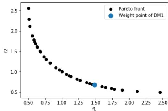
Figure 3.2: A Pareto front for the given functions. The blue point is the point which is obtained from the weight of decision maker one.
